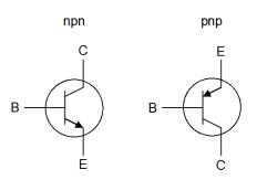
The BJT can be used as a simple switch or as an amplifier. The operation is always controlled by the baseemitter junction  $J_e$  which is forward biased, while if reverse biased the BJT is turned off. The base-collector  $J_c$  junction is forward biased for use as a switch, while it is reverse biased for use as an amplifier.
