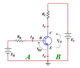
We have the input mesh (A) characterized by  $V_{BE}$  and  $I_B$ , and the output mesh (B) characterized by  $V_{CE}$  and  $I_C$ .
