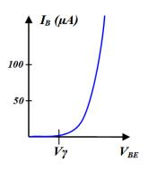
The input characteristic represents the trend of the current  $I_B$  as a function of the  $V_{BE}$  therefore we refer to the junction  $J_e$  between the base and the emitter, directly biased. The characteristic is that of a diode with threshold voltage  $V\gamma$ =0.7V, so  $V_{BE}$ =0.7V when the BJT is directly biased.
