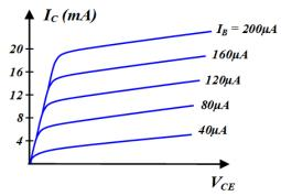
The output characteristics represent the trend of the current  $I_C$  as a function of the  $V_{CE}$  for constant values of  $I_B$ . It is therefore a family of curves.
